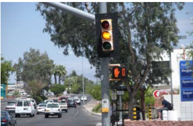
Pedestrians are assisted with crossing the intersection through the use of pedestrian countdown signals.
