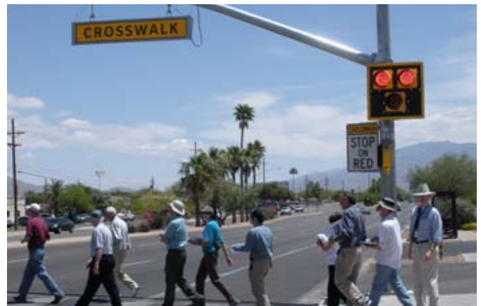
The pedestrian auditors walking within a crosswalk that has a HAWK signal at 8200 East Broadway Boulevard.
