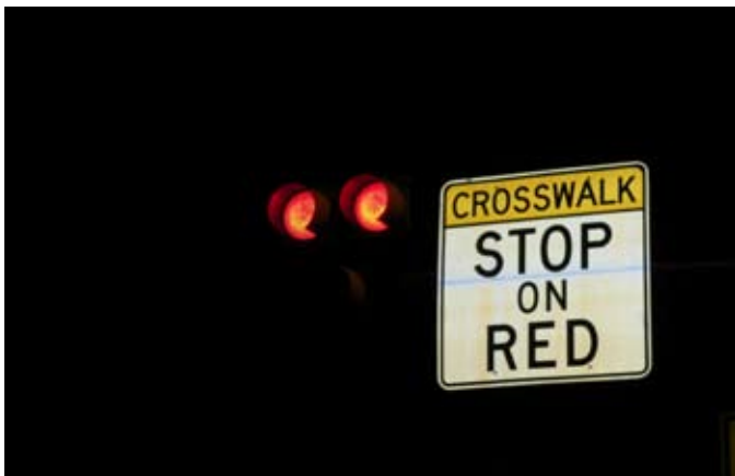
Nighttime illumination sign at a HAWK signal.
